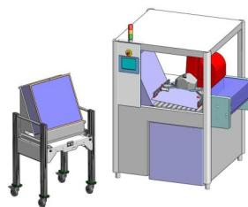
MAP650 unloads from cassettes with automatic format adjustment, double sheet detection and centering device. The integrated mylar peeler is equipped with mylar tear detection and re-peeling function. First UK customers orders have already been placed.
